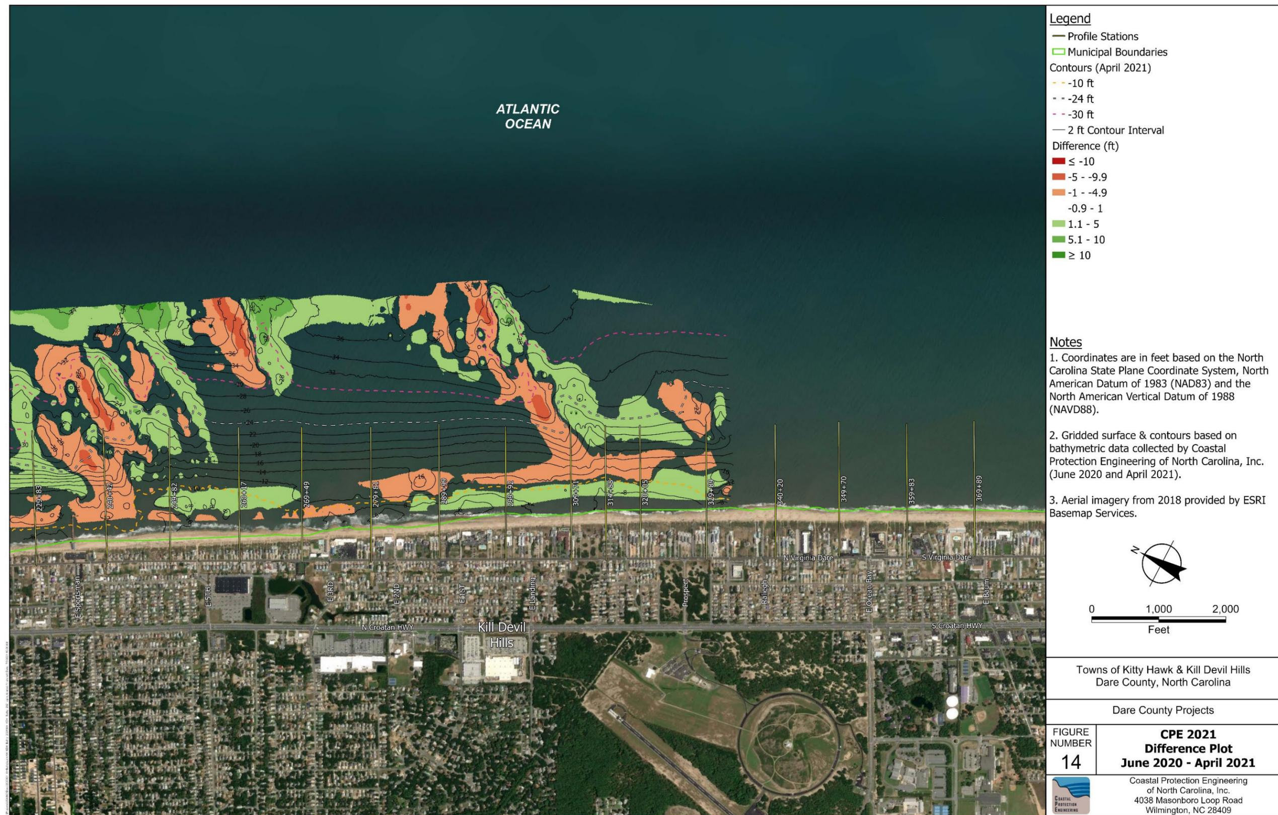
Figure 14. Map Illustrating the Changes in the Measured Depth between the June 2020 CPE and April 2021 Bathymetric Surveys Conducted by CPE between Baseline Stations 229+83 and 329+89
