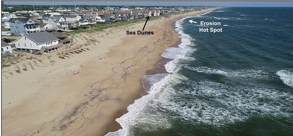
**Figure 6. Drone Image of Erosional Hot Spot at Station 149+99 from July 16, 2020**
