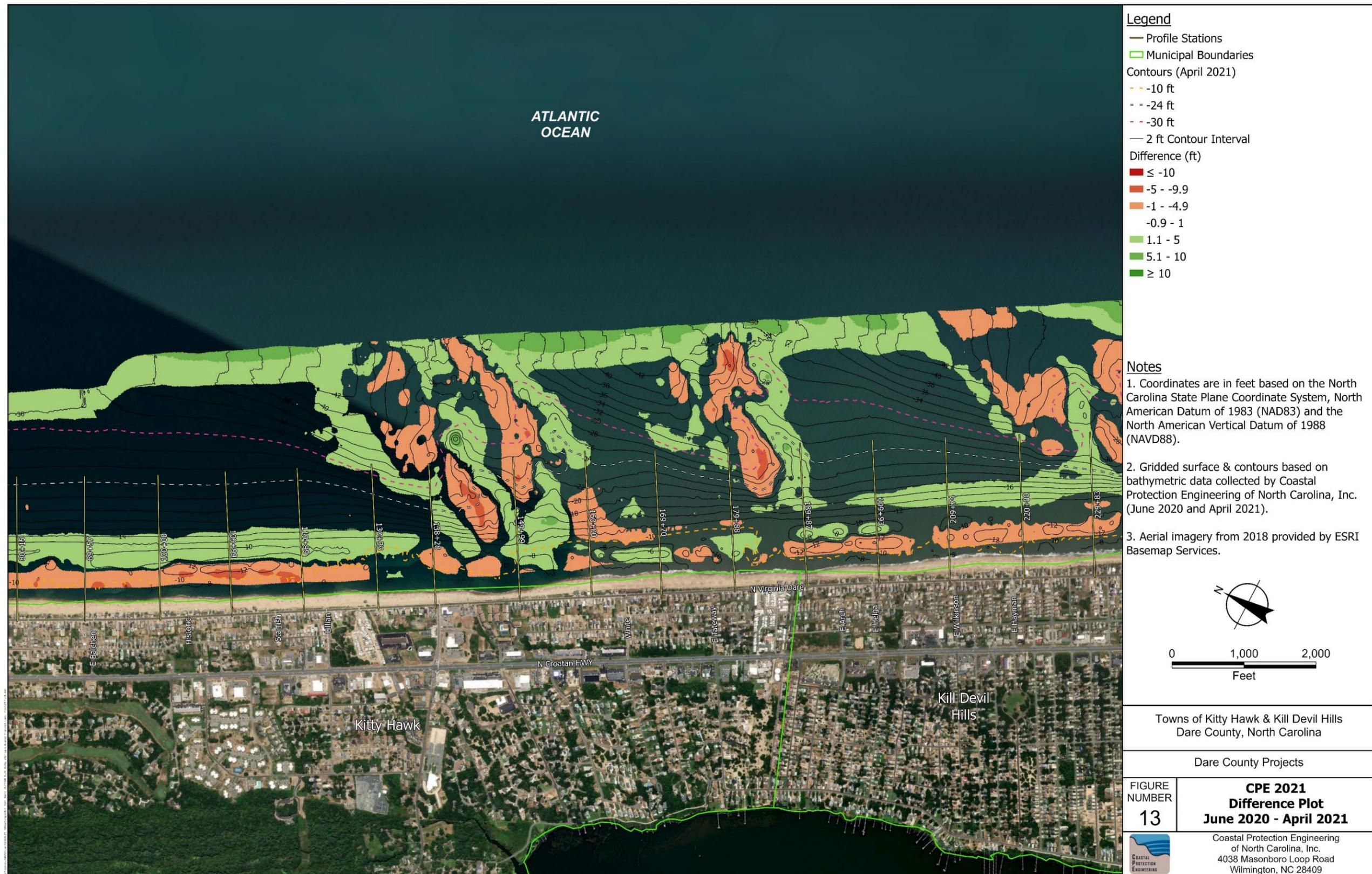
Figure 13. Map Illustrating the Changes in the Measured Depth between the June 2020 CPE and April 2021 Bathymetric Surveys Conducted by CPE between Baseline Stations 80+15 and 229+83
