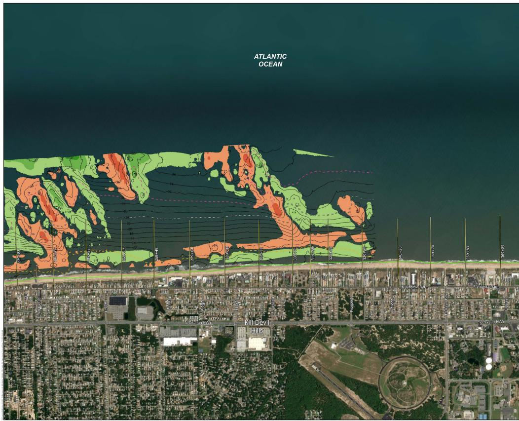
Figure 14. Map Illustrating the Changes in the Measured Depth between the June 2020 CPE and April 2021 Bathymetric Surveys Conducted by CPE between Baseline Stations 229+83 and 329+89
