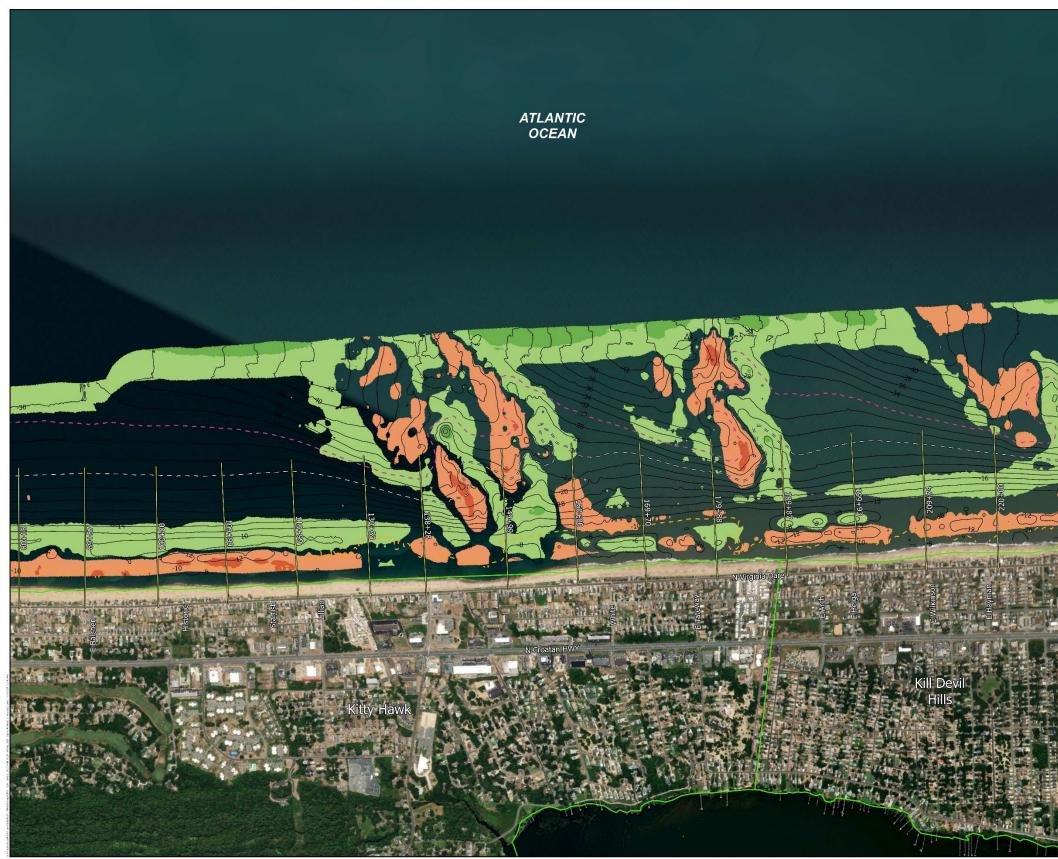
Figure 13. Map Illustrating the Changes in the Measured Depth between the June 2020 CPE and April 2021 Bathymetric Surveys Conducted by CPE between Baseline Stations 80+15 and 229+83
